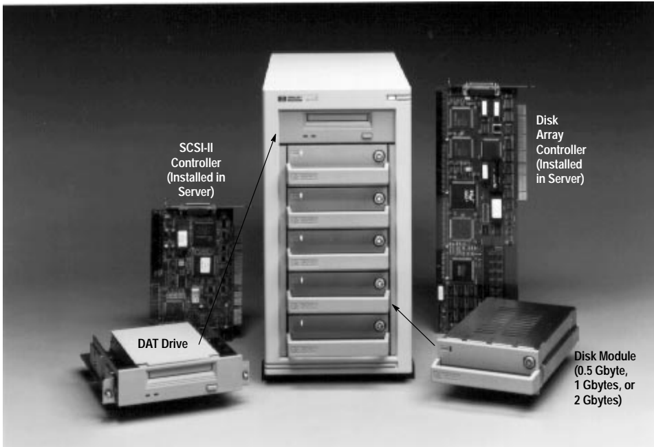
Fig. 2. The components of an HP storage system. The SCSI-II controller, the disk array controller, and the disk module make up the HP Disk Array.
